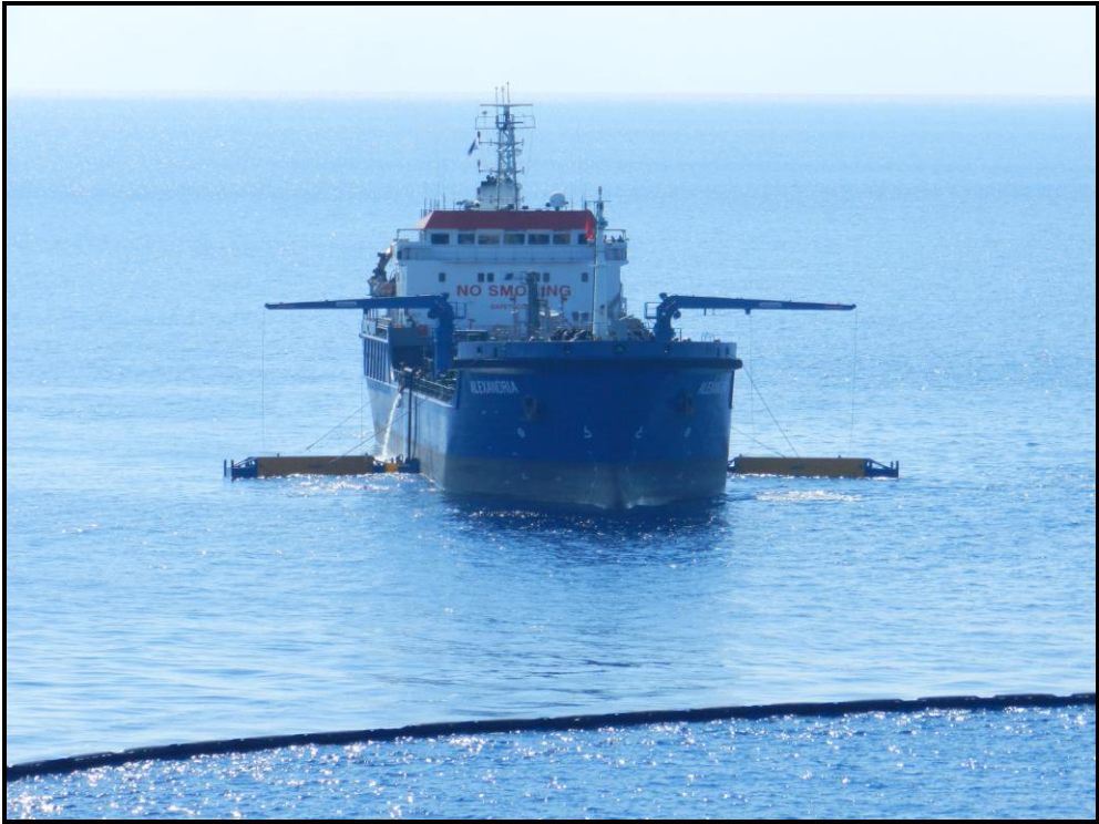
Oil Recovery Vessel “ALEXANDRIA” with deployed rigid sweeping arms
