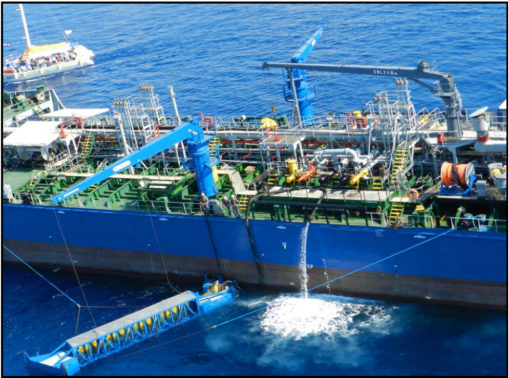
Rigid sweeping arm and clean water discharge
