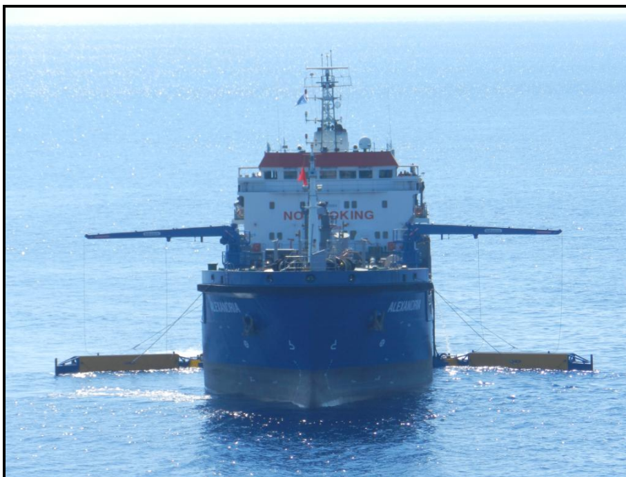
“ALEXANDRIA” operating with deployed rigid sweeping arms
