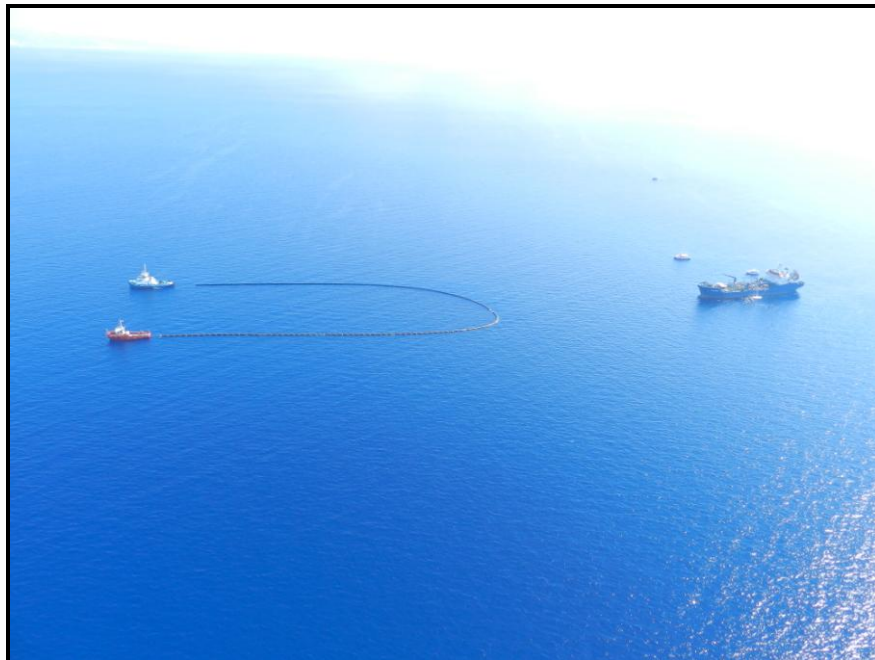
Boom deployed in “U” form with an open end
